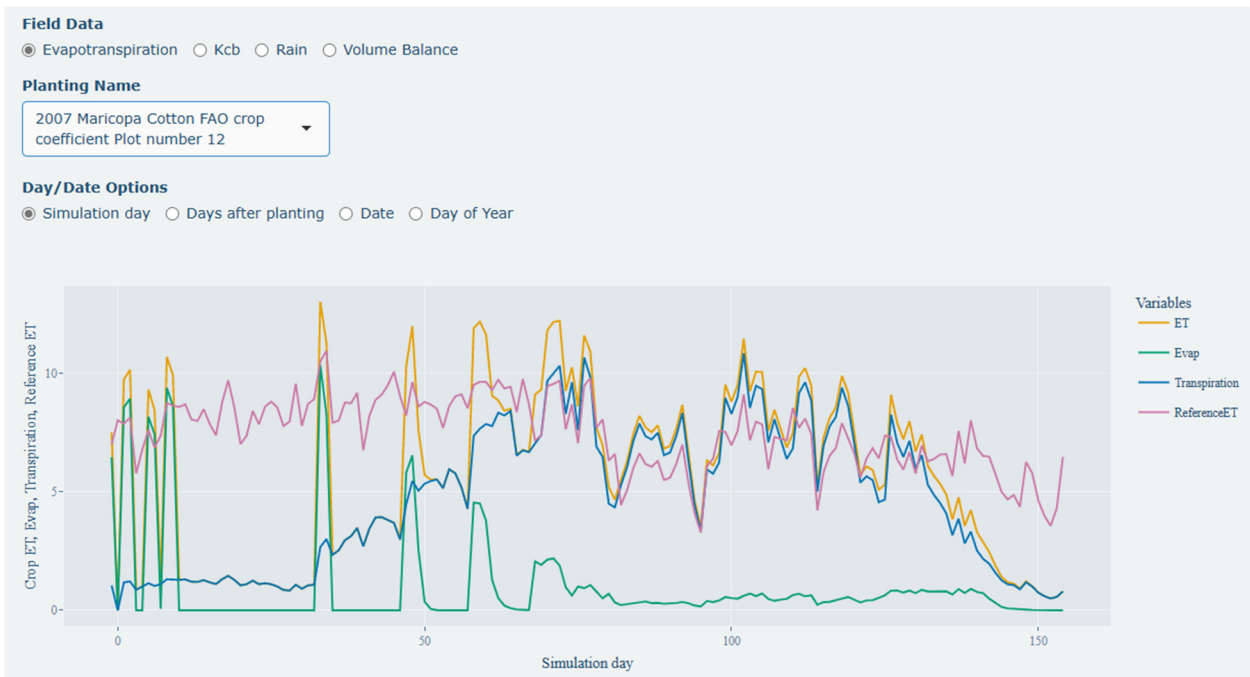
Figure 8. WINDS (Water-use, Irrigation, Nitrogen, Drainage, and Salinity) model simulation ( https://vis.datascience.arizona.edu/WINDS/ Please wait for web page to load) of crop ET, evaporation, transpiration, and reference ET for the FT (FAO) treatment, plot 12, in the 2007 cotton experiment in Maricopa, Arizona.
